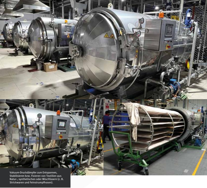
Vacuum pressure steamer for relaxing, stabilising or turn-fixing of textiles made of natural, synthetic or blended fibres (f. ex. knitted goods and tights).
